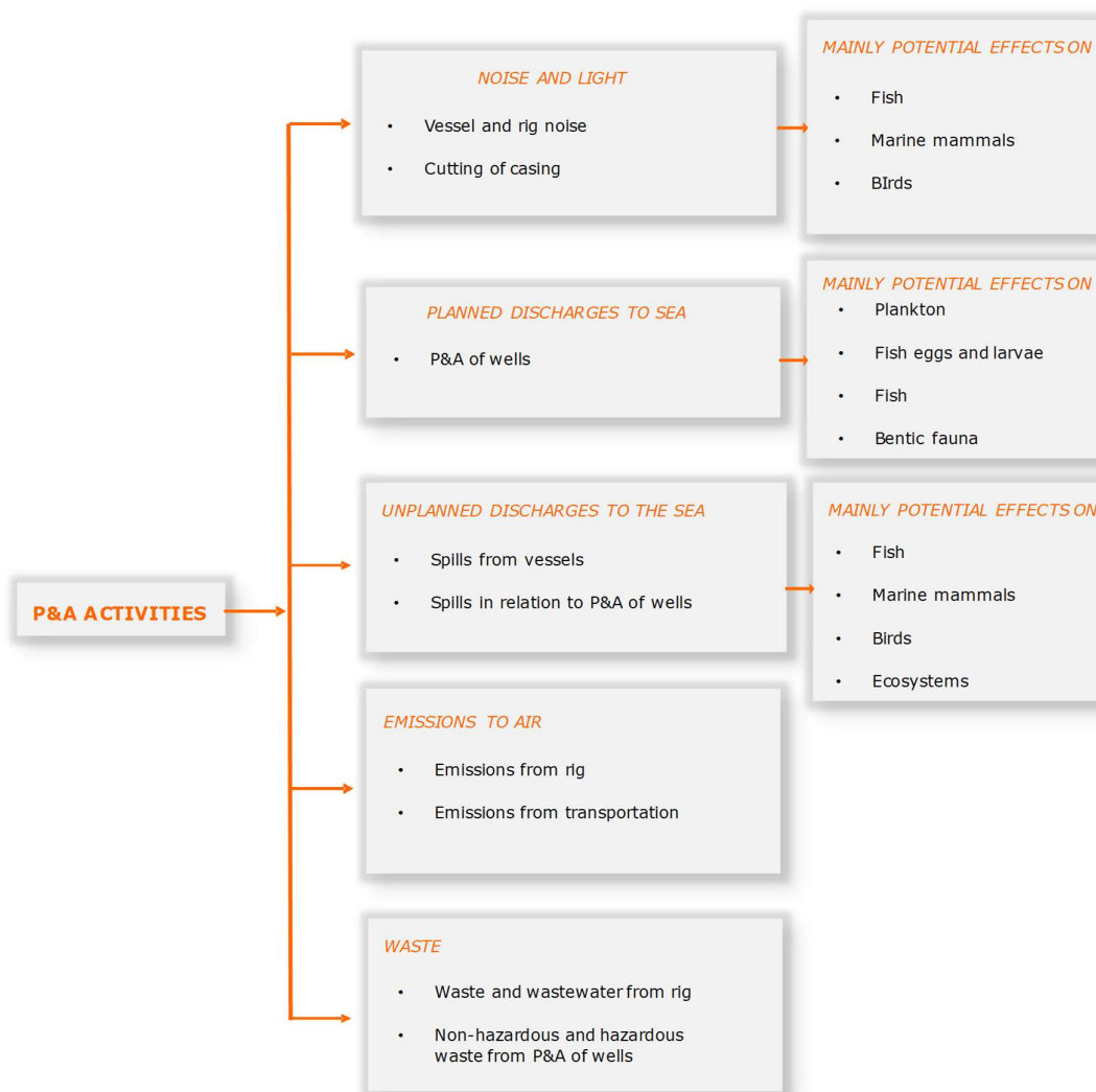
Figure 3-3 Overview of potential environmental impacts from P&A activities and effects on environmental components.
