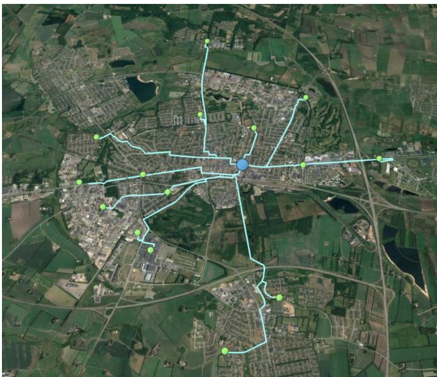
Exhibit 4.15: Illustrative example of the calculation of routes between network nodes [Source: Axon Consulting]
