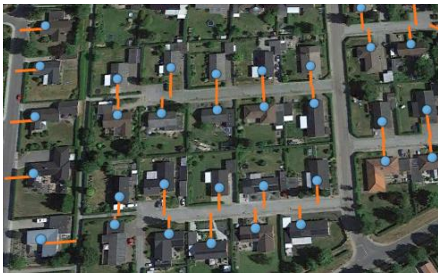
Exhibit 4.9: Projections of the buildings on the road sections [Source: Axon]
