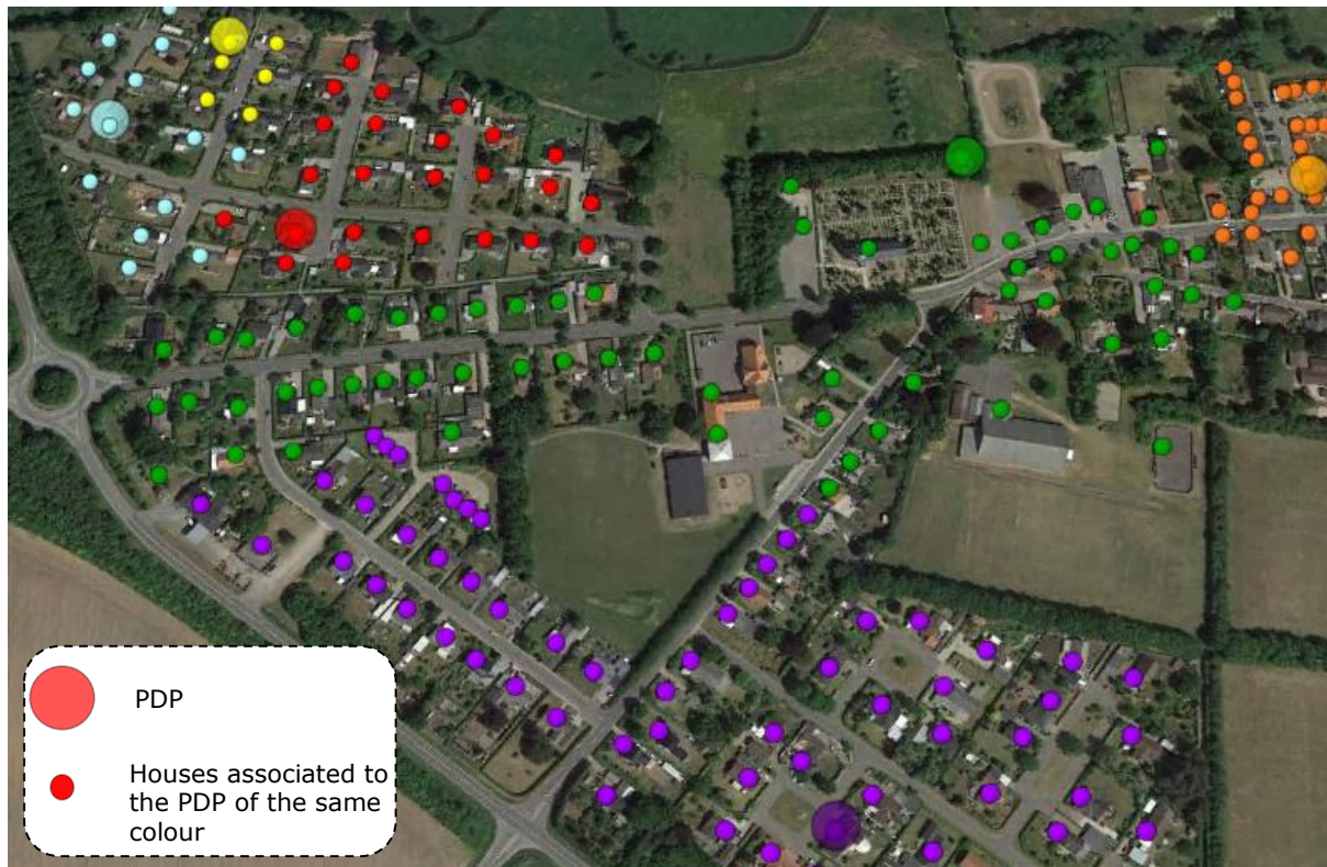
Exhibit 4.10: Example of PDP areas, where each colour represents a different PDP area [Source: Axon Consulting]
