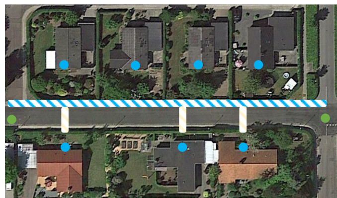
Exhibit 4.39: First option for the second trench in each section [Source: Axon Consulting]
